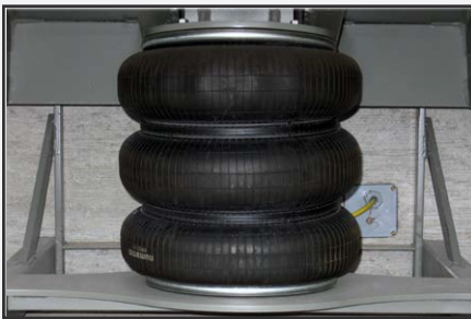
Steel belted rubber bellows system uses compressed air to raise platform.
