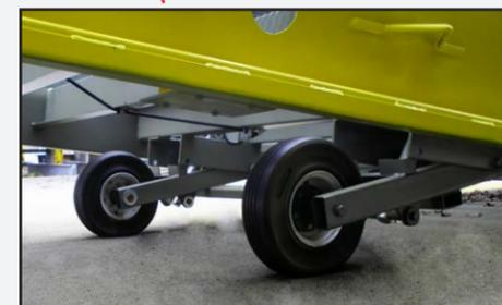
Heavy duty axle assembly with 18" industrial solid rubber tires adds a high level of mobility to the yard ramp for easy positioning. Note: axle assembly can be removed or raised for permanent dock ramp installations.
