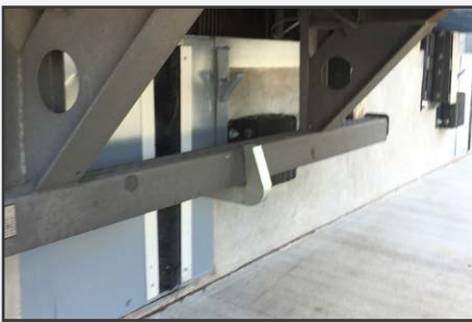
The PowerHook seeks, finds, and secures a trailer's RIG to the dock.
