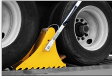
The chock system is installed with an articulated arm and ground plate to lock the chock in position.
