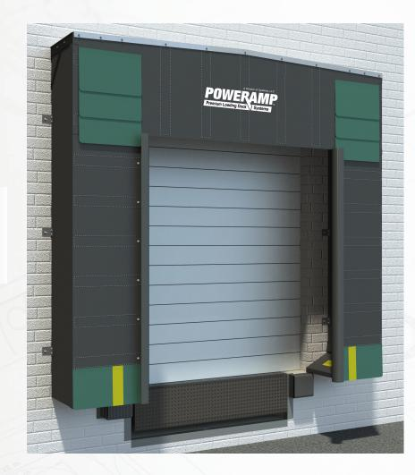
GS Series Dock Shelter—engineered for use with swing-door trailers, the GS Dock Shelter seals the air and light gaps at door hinges while still allowing full access into the trailer. This shelter provides maximum dock protection while minimizing pressure on the building wall. Utilizing foam side pads in its construction, the shelter is capable of compressing and bending out of the way of a truck that approaches the dock off-center preventing costly repairs.
