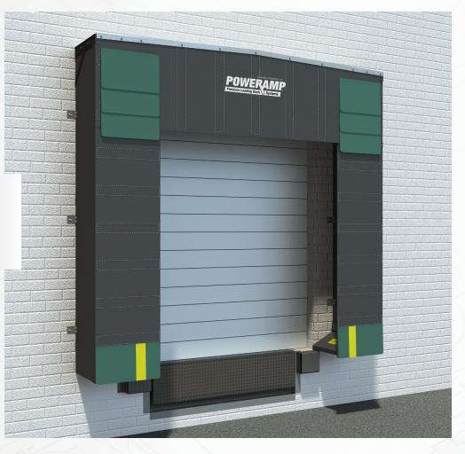
Soft Sided Series Dock Shelter—provides maximum dock protection and full access to trailers while minimizing pressure on the building wall. The Dock Shelter has soft foam sides for added flexibility and is able to compress and bend out of the way of a truck that approaches the doorway off-center or misaligns with the dock. It is designed to be pliable to prevent damage, downtime and costly repairs.
