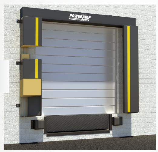
Full Pad Series Dock Seal—accommodates larger doors and features foam-filled head and side pads that provide a positive seal. The tight, energy-efficient seal between the trailer and dock wall protects the dock from inclement weather, dirt and insect infiltration.
