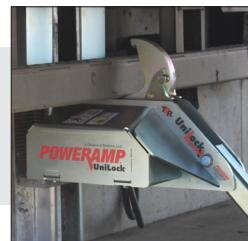
The TPR hook rotates up to engage the RIG and secure the trailer to the loading dock.
