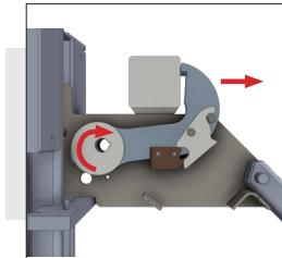
Advanced cam design rotates hook away from RIG first to release pressure from "RIG Wedge."
