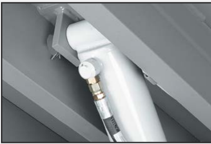
Inverted Piston Style Hoist Cylinder.
