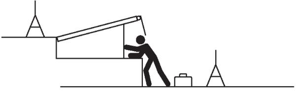
Always post safety warnings and barricade the work area at dock level and ground level to prevent unauthorized use of the equipment before maintenance is complete.
