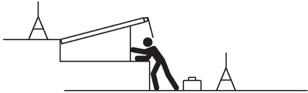
Always post safety warnings and barricade the work area at dock level and ground level to prevent unauthorized use of the equipment before maintenance is complete.
