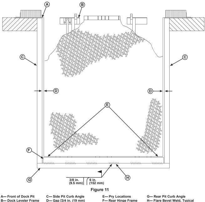
8. With rear hinge frame angle (F) tight against rear pit curb angle (G), perform/check the following:
