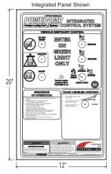
**INSTALLATION:** Requires mounting of locking unit, control panel, exterior lights and signs in strict accordance with Poweramp installation instructions. Mechanical installation is recommended to be performed only by authorized Poweramp Representative.
